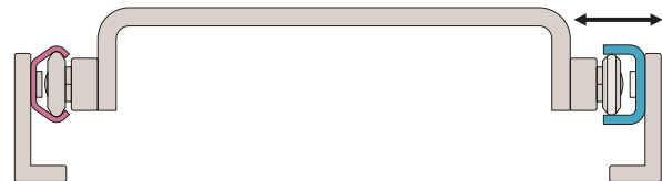
T and U rail allows for misalignment
