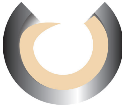
Self-lubricating with teflon liner
